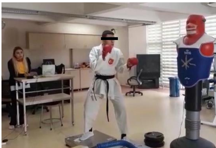
Picture 1. Repetitive kick force and duration test (Source: Captured by authors.)
