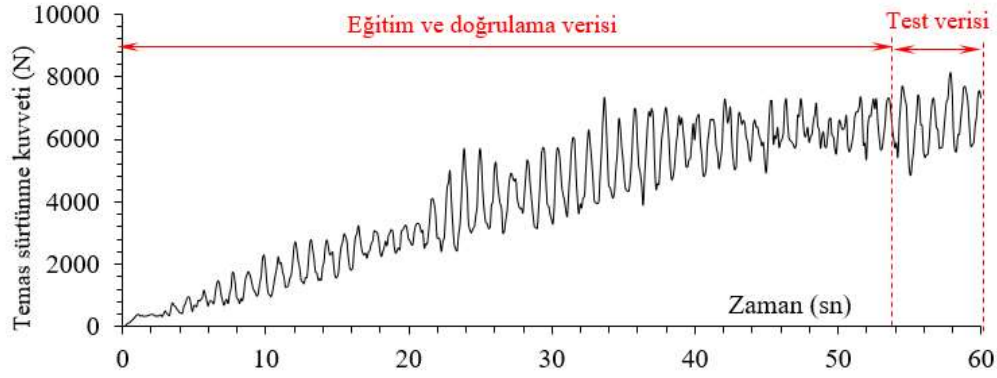
Figure 4. Time series data of contact friction force from the simulation and data portions
