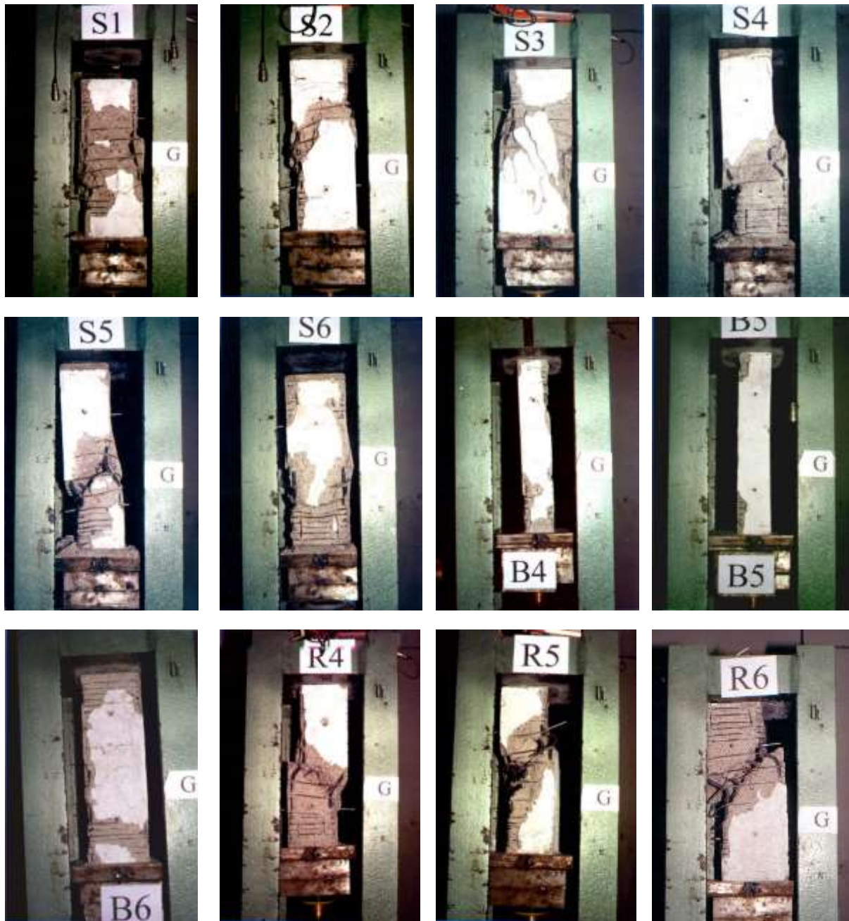
Figure 5. Damage distribution of specimens after test
