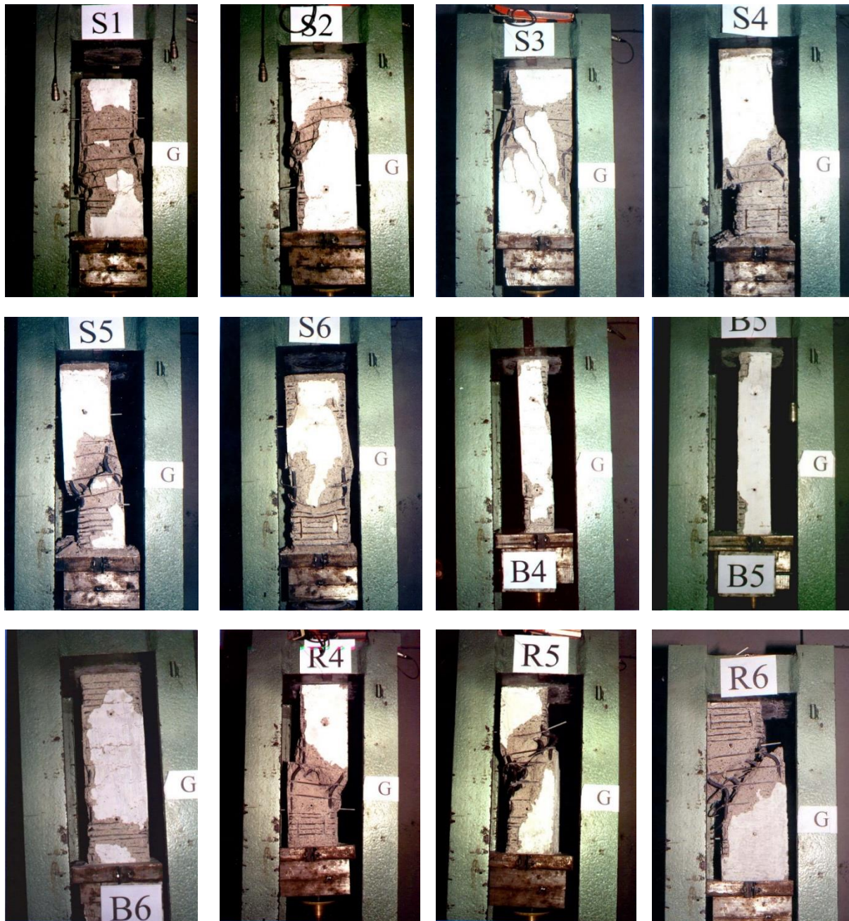
Figure 5. Damage distribution of specimens after test
