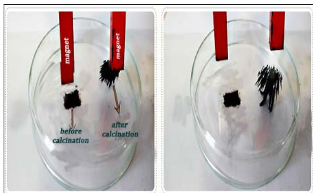
Figure 9. The interaction of cobalt ferrite nanoparticles with magnet before and after calcination.
