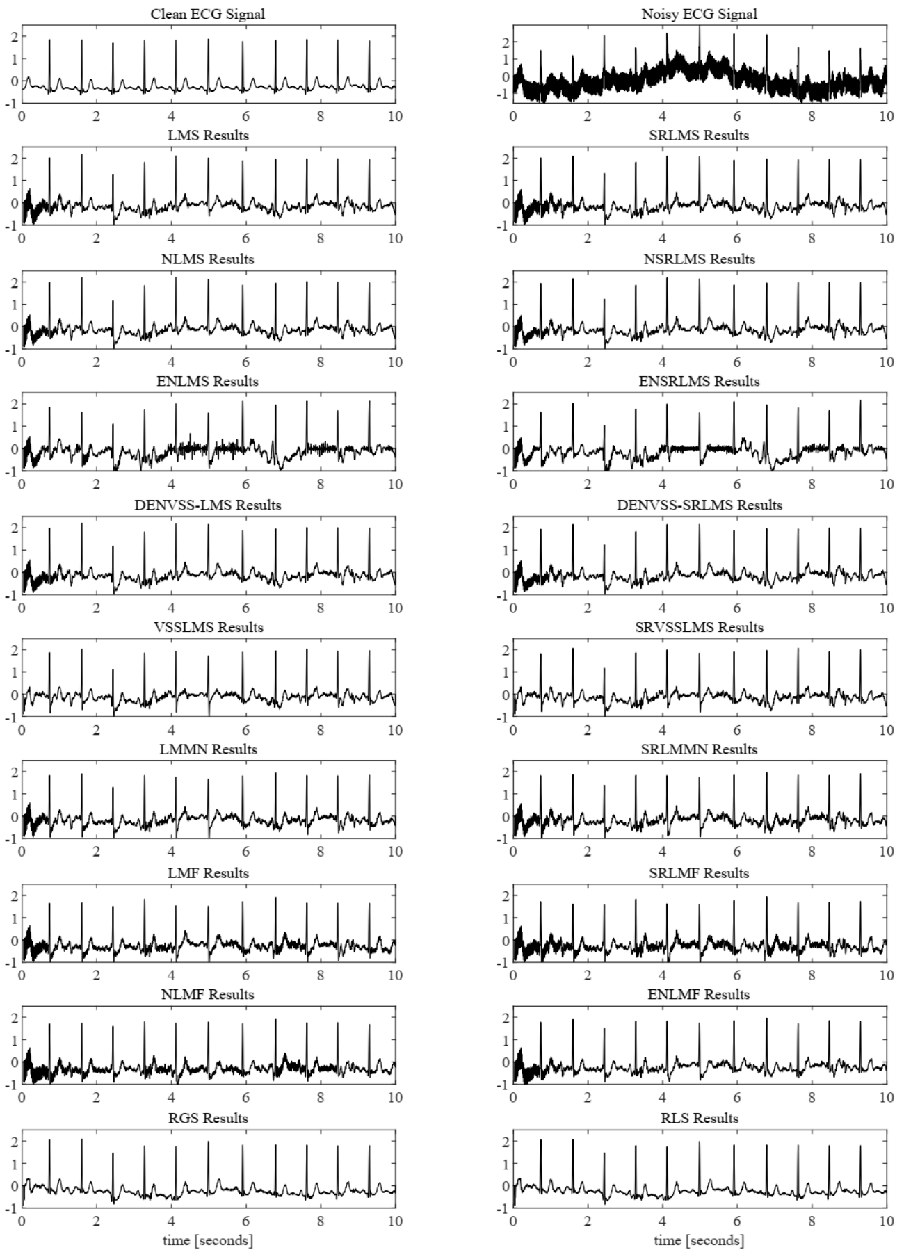
Figure 3. Comparison of the denoised ECG waveforms obtained by cancellation of mixed noise.
