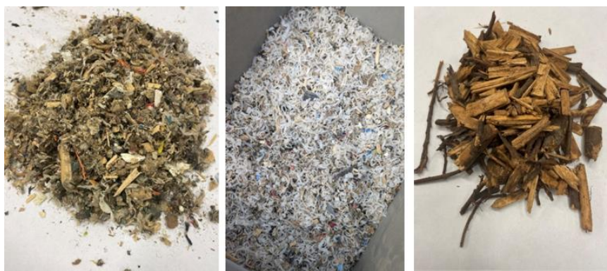
Figure 1. Photos of SRF (left), waste HDPE (middle), and Willow Wood (right) samples
