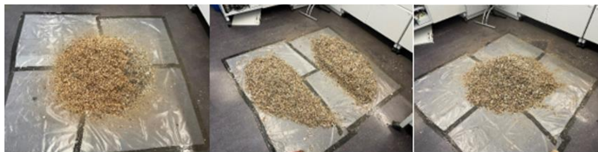
Figure 2. Photos of mixing samples by cone and quartering
