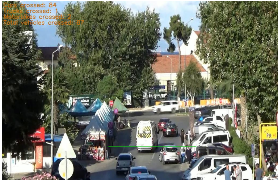
Figure 7. Vehicle counting using YOLOv9.
