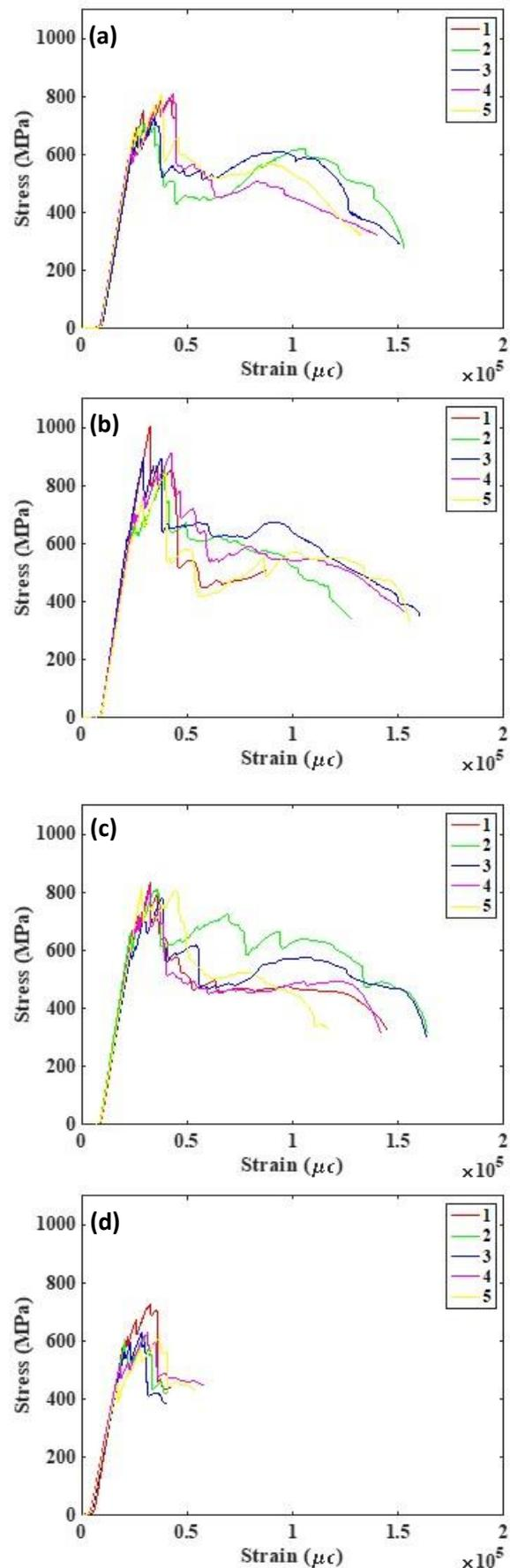
**Figure 4:** Stress-strain plot of samples, a) tested in 20 mm/min (Group A), b) tested in 40 mm/min (Group B), c) tested in 60 mm/min (Group C), d) tested in 2 mm/min (Group D)
