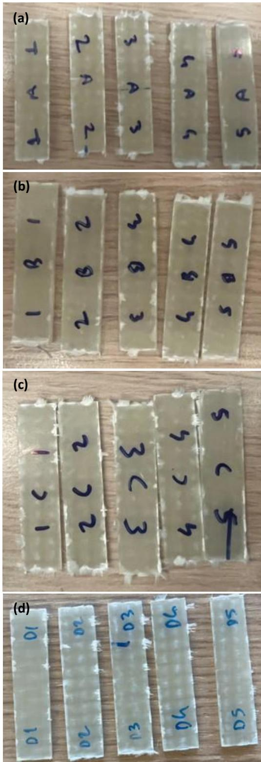
Figure 2: Specimens just before the 3-point bending test
