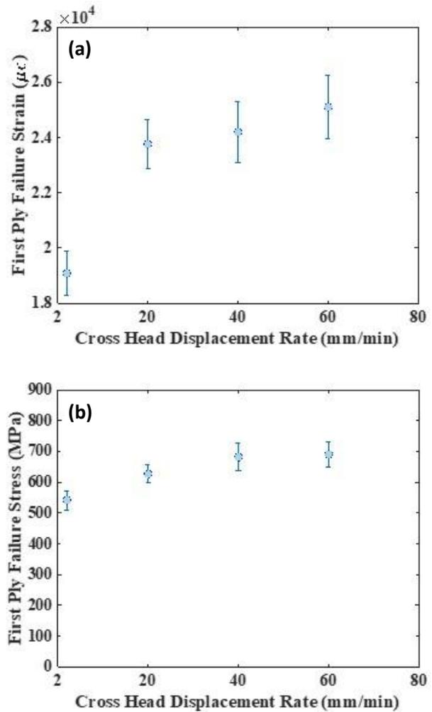
**Figure 6:** First ply failure, a) Strain, b) Stress
