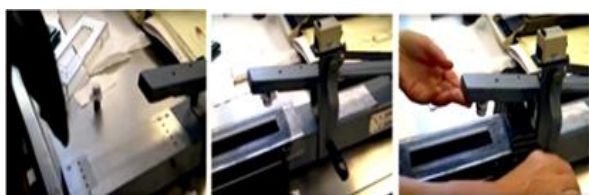
Figure 1. Dry rubbing fastness test.
