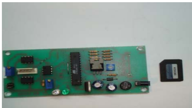
Fig.5. Constructed electronic circuit board and MMC memory card.
