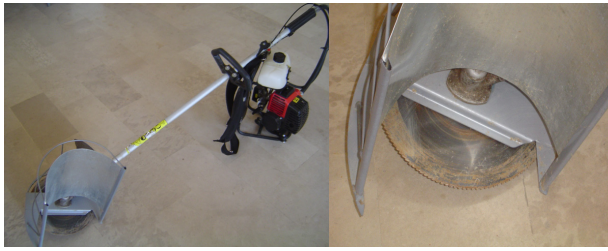
Fig. 7. Final form of used rice reaper with designed head
