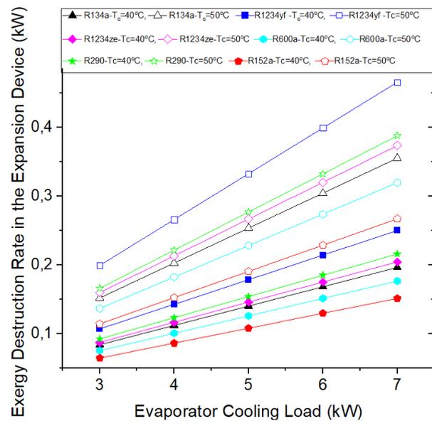
Figure 12. The rate of exergy destroyed in the expansion device vs. evaporator cooling load
