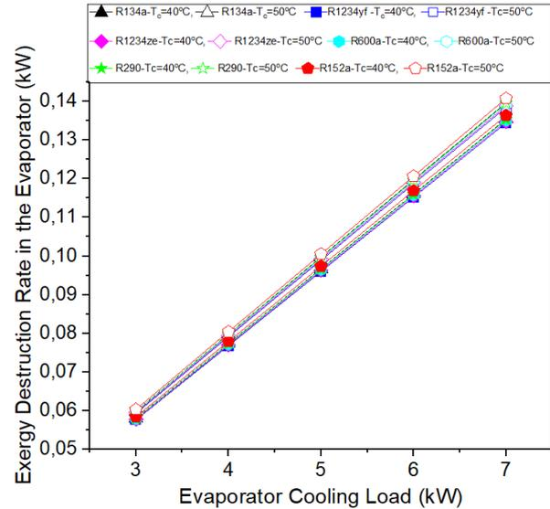
Figure 11. The rate of exergy destroyed in the evaporator vs. evaporator cooling load
