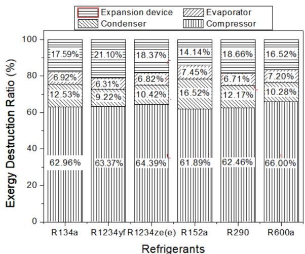
Figure 15. The percent distribution of the destroyed exergy in the elements of the MAC system for  $Q_{evap} = 5\text{ kW}$ ,  $T_{evap} = -2\text{ }^{\circ}\text{C}$  and  $T_{cond} = 50\text{ }^{\circ}\text{C}$
