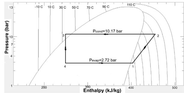
Figure 3. P-h diagram of the refrigeration cycle of the MAC system for R134a
