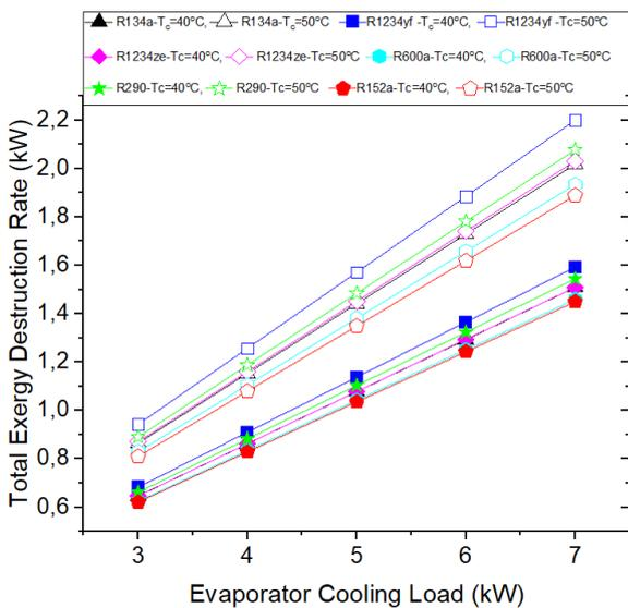
Figure 13. The rate of total exergy destroyed in the MAC system vs. evaporator cooling load
