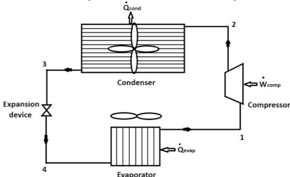
Figure 1. Schematic view of the MAC system
