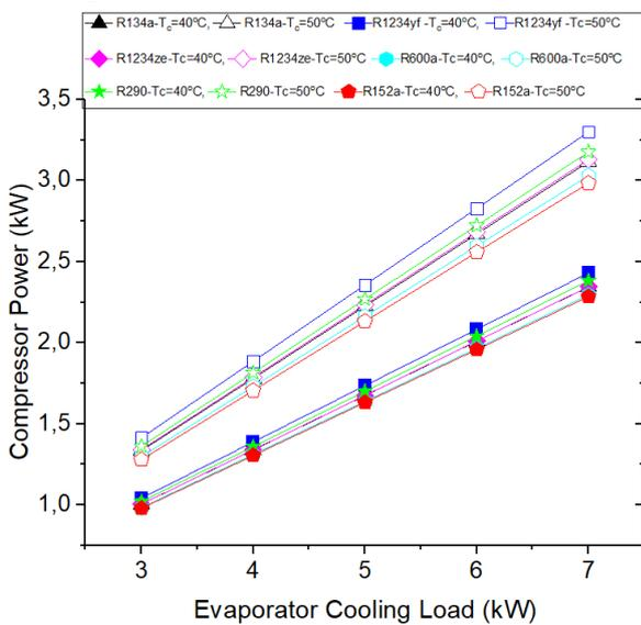
Figure 5. Compressor power vs. evaporator cooling load
