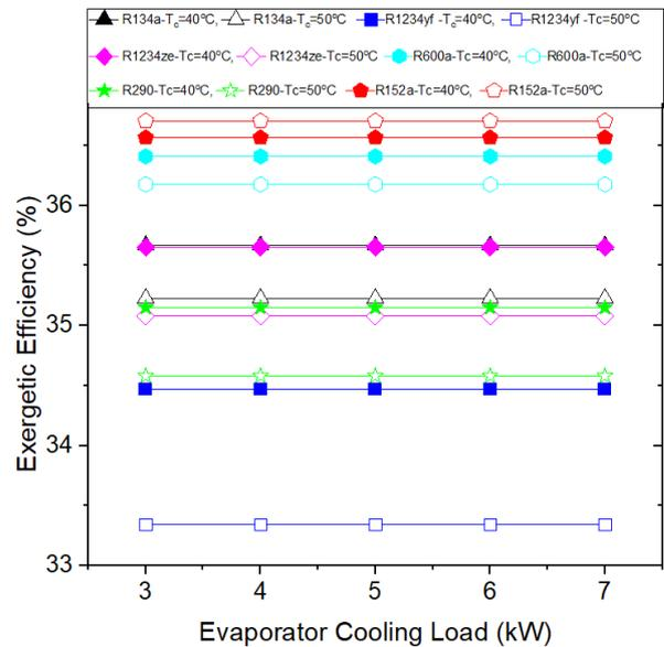
Figure 14. Exergetic efficiency of the MAC system vs. evaporator cooling load
