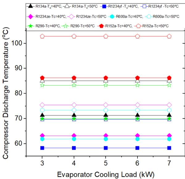
Figure 8. Compressor discharge temperature vs. evaporator cooling load
