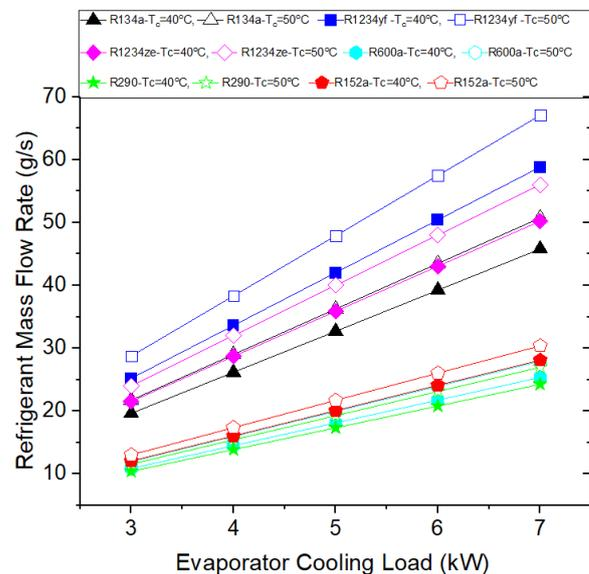
Figure 4. Refrigerant mass flow rate vs. evaporator cooling load
