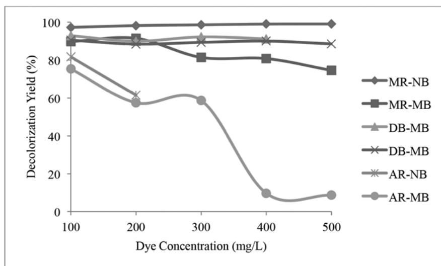
**Figure 2.** The effect of dye concentration on decolorization of textile dyes in nutrient broth and molasses media at  $30^\circ\text{C}$  at 48 h. (MR-NB: Maxillon Red-Nutrient Broth, MR-MB: Maxillon Red-Molasses Medium, DB-NB: Doracryl Blue-Nutrient Broth, DB-MB: Doracryl Blue-Molasses Medium, AR-NB: Astrozon Red-Nutrient Broth, AR-MB: Astrozon Red-Molasses Medium)
