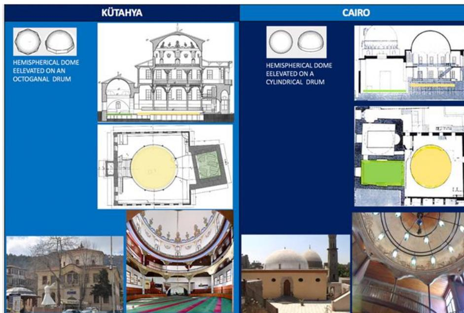
**Figure 11.** (a) Kütahya- Section and plan drawings [1] Exterior and interior photos [9]
