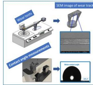
Figure A: The wear and contact angle measurements of ZrO<sub>2</sub> coated CP-Ti material
