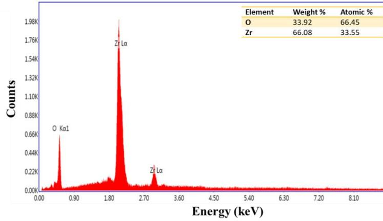
**Figure 4.** EDS analys result of ZrO<sub>2</sub> film (ZrO<sub>2</sub> filminin EDS analiz sonucu)
