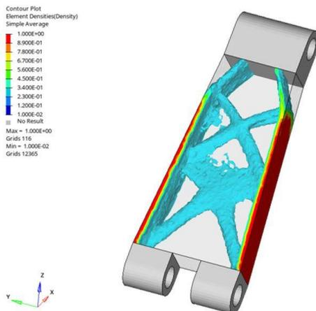
Figure 6. Topology optimization result of bending condition
