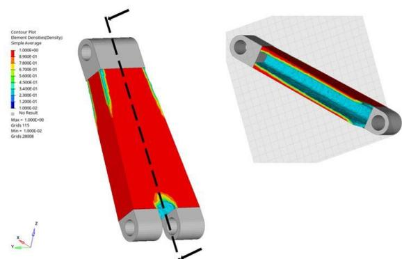
Figure 8. Topology optimization result of EEWC Method
