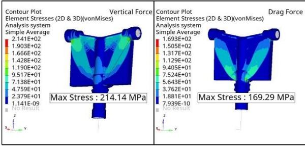
**Figure 16.** Optimized Trunnion Von-Mises stress results according to the EEWC method
