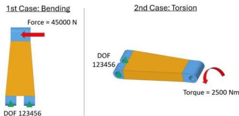
**Figure 5.** Loading and boundary conditions
