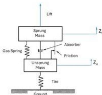
**Figure 3.** Schematic representation of a single landing gear [10]
