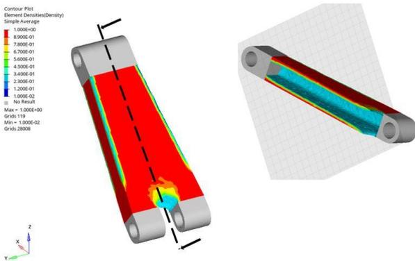
**Figure 9.** Topology optimization result of PWC Method
