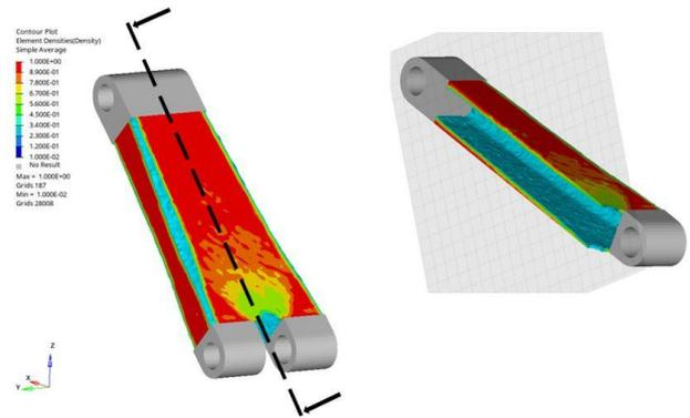
Figure 7. Topology optimization result of torsion condition
