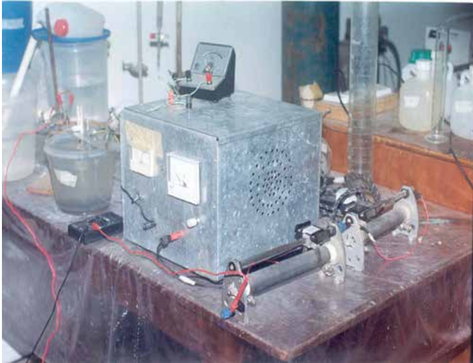
Figure 2b. Laboratory setup of a two electrode electrochemical treatment process
