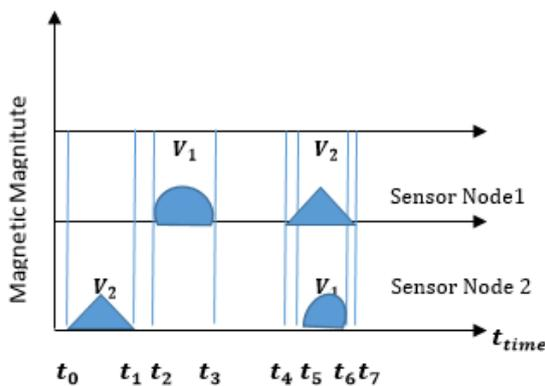
Figure 8. Determining the direction of the vehicles
