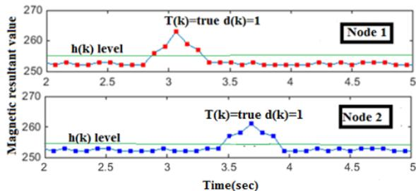
c) Detection of the vehicle direction, from left to right (Adaptive threshold algorithm)
