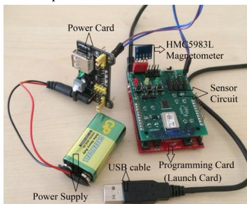
Figure 3. Sensor circuit designed for vehicle direction detection
