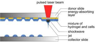
Figure 4. Schematic laser-assisted bioprinting setup [17].
