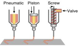
Figure 3. Microextrusion bioprinting systems [2].
