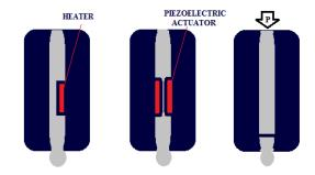
Figure 2. Schematic representation of inkjet printer methods. The figure on the left shows thermal inkjet bioprinter. The figure in the middle shows piezoelectric bioprinter. The figure on the right shows mechanical inkjet bioprinter
