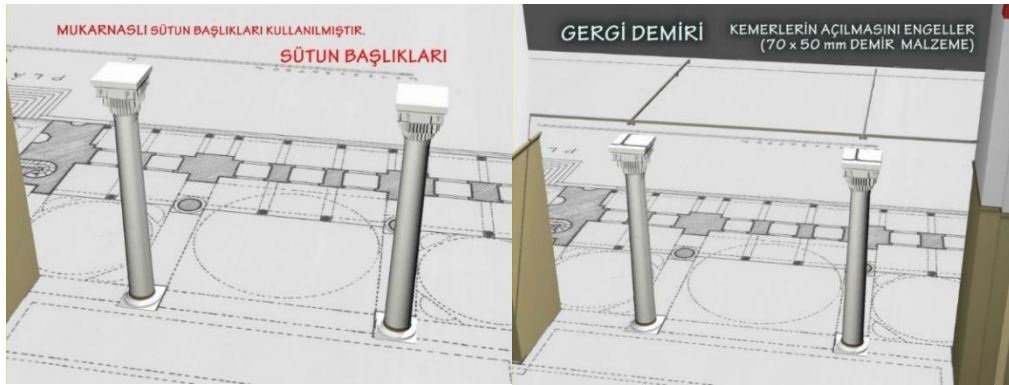
Figure 13. Animation frames: Mucarnassed column heads and tension bars preventing the arches from opening
