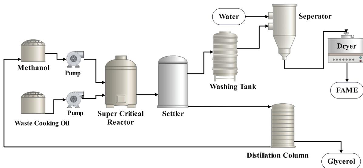
Figure 6. Schematic of biodiesel production from WCO by supercritical methanol process.
