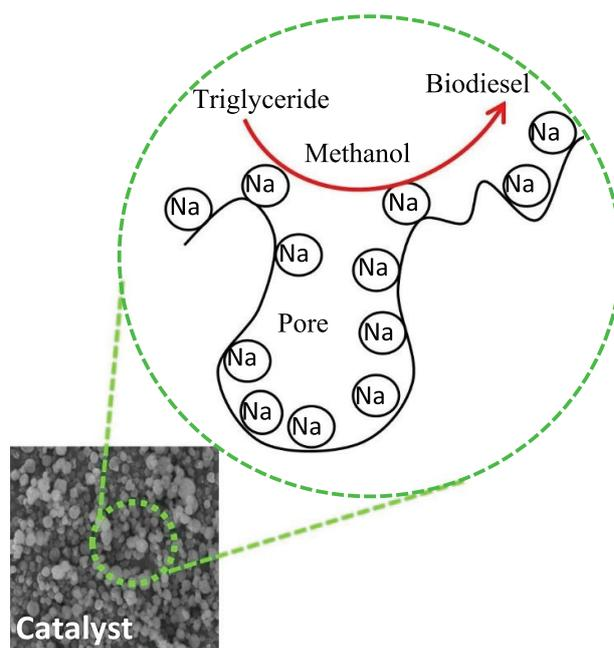
**Figure 12.** Schematic representation of triolein transesterification for biodiesel production using Na-treated zeolite catalyst.
