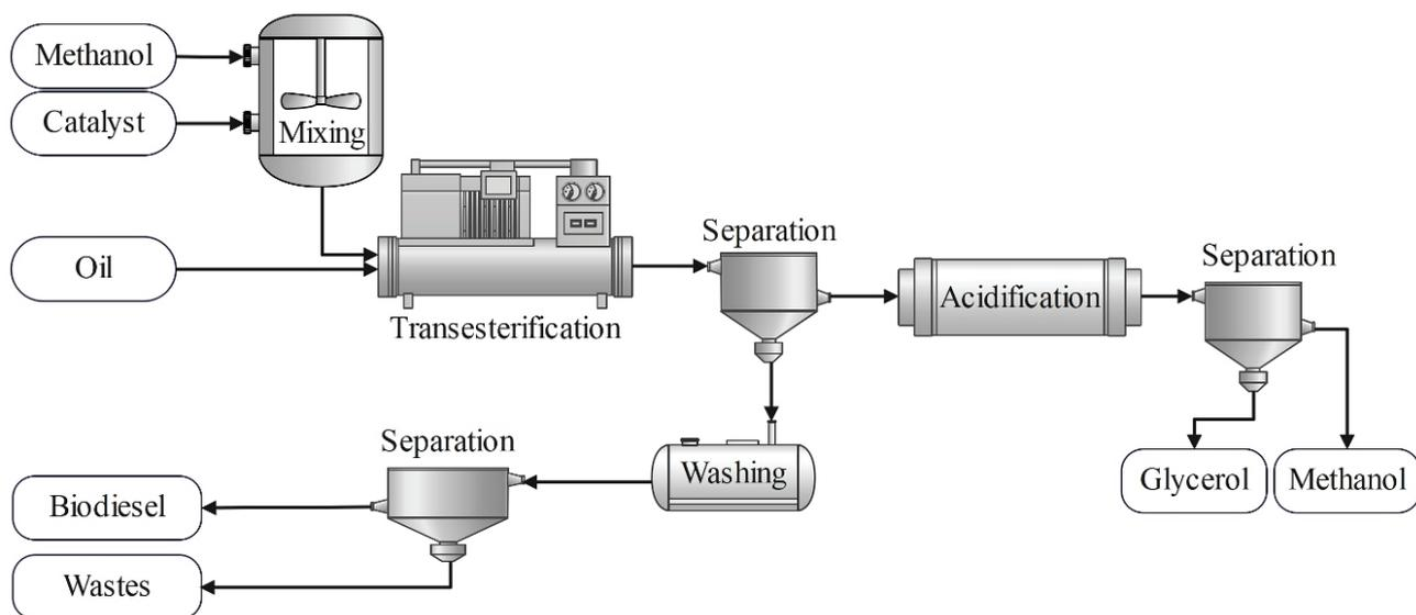
Figure 8. Schematic of biodiesel production via transesterification process.
