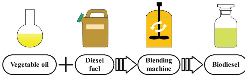
Figure 5. Schematic of blending (dilution) method for biodiesel production.
