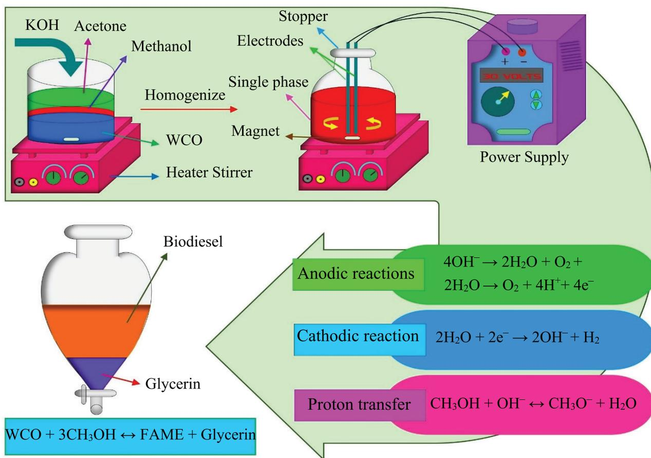
Figure 9. The schematic representation of the electrolysis process for biodiesel production using waste cooking oil (WCO) transesterification.
