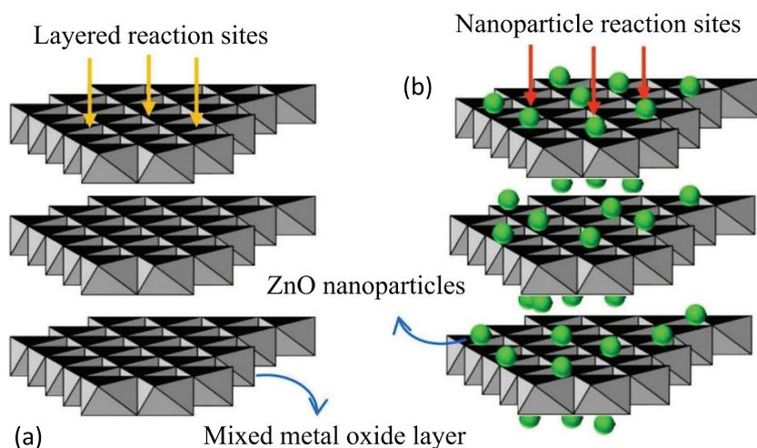
**Figure 13.** Schematic representation of active sites in (a) co-precipitated ZnMgAl, and (b) Zn/MgAl(O) [170] [Open Access].
