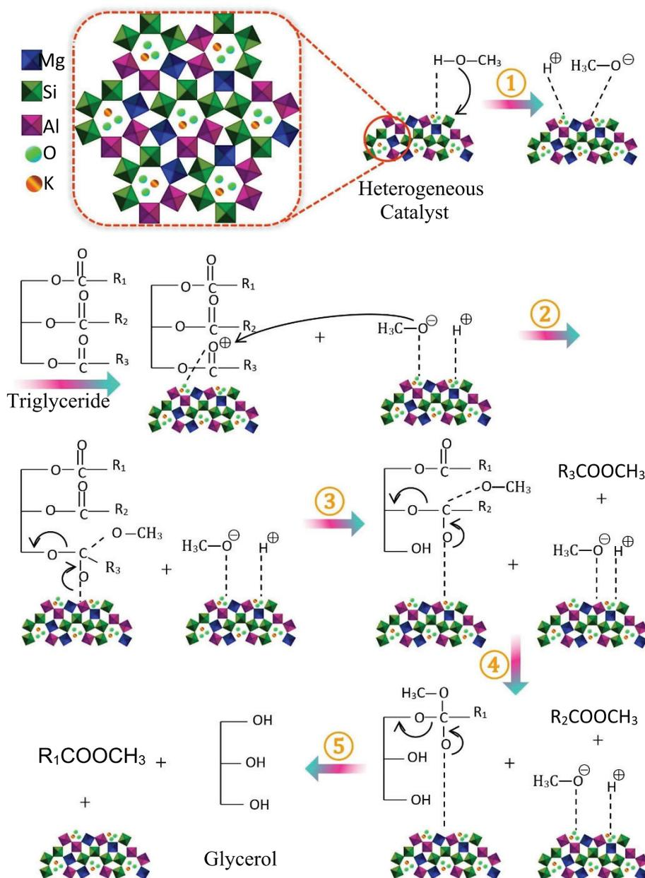
**Figure 11.** The transesterification mechanism for biodiesel production from sunflower oil using MgAl-LDH based potassium/geopolymer.
