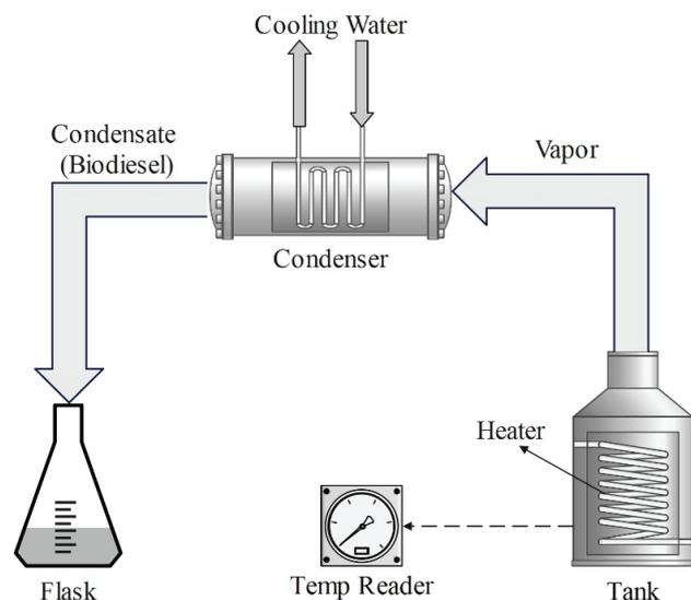
**Figure 7.** Schematic of biodiesel production by pyrolysis of WCO.
