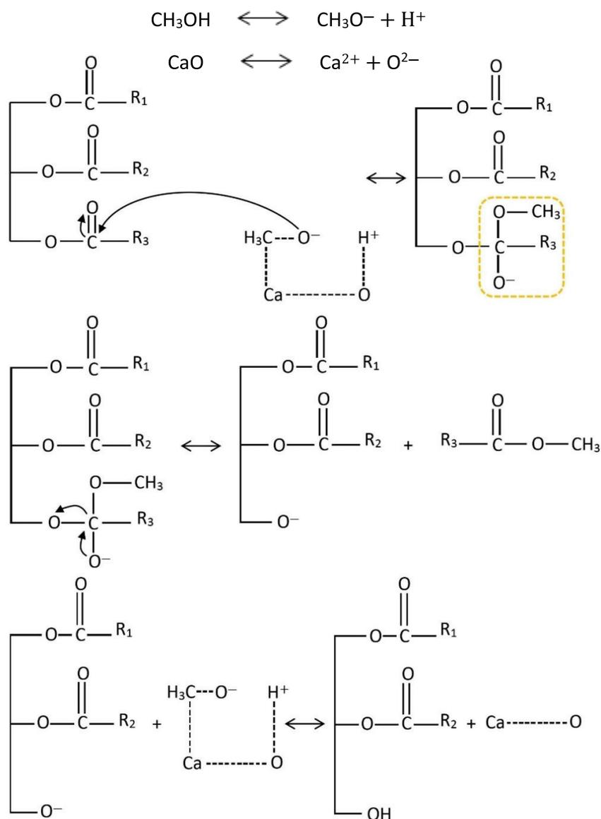
Figure 10. Triglyceride transesterification mechanism using CaO as catalyst.
