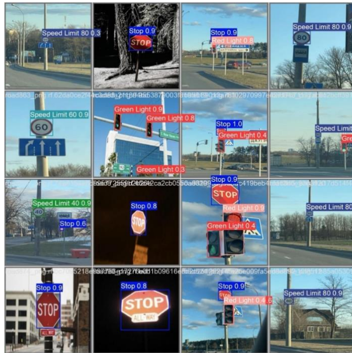
Figure 13. Confidence values for the test data of the off-vehicle model (SelfDriving Car, 2023)
