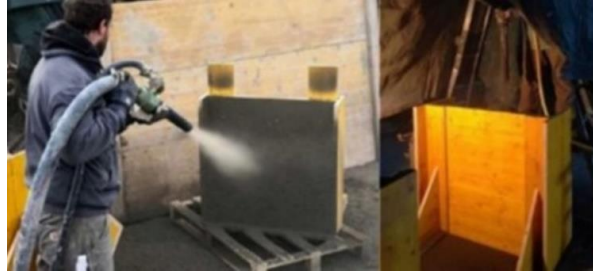
Figure 2. Spraying process in single-sided (left) and double-sided (right) moulds (Curto et al., 2020:3).
