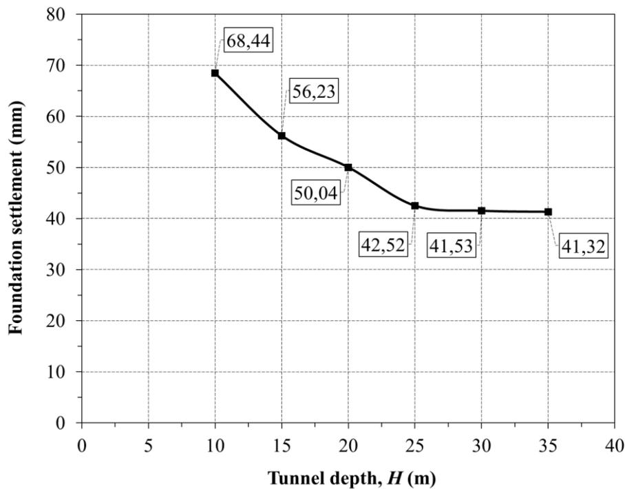
**Figure 6.** Tunnel depth-foundation settlement curve
