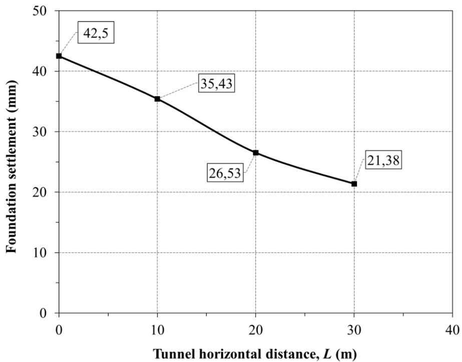
**Figure 10.** Tunnel epicentric distance-foundation settlement curve
