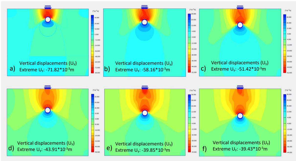
**Figure 5.** General presentation of vertical displacements ( $U_y$ ) a) for  $D=10$  m,  $H=10$  m, b) for  $D=10$  m,  $H=15$  m, c) for  $D=10$  m,  $H=20$  m, d) for  $D=10$  m,  $H=25$  m, e) for  $D=10$  m,  $H=30$  m, f) for  $D=10$  m,  $H=35$  m
