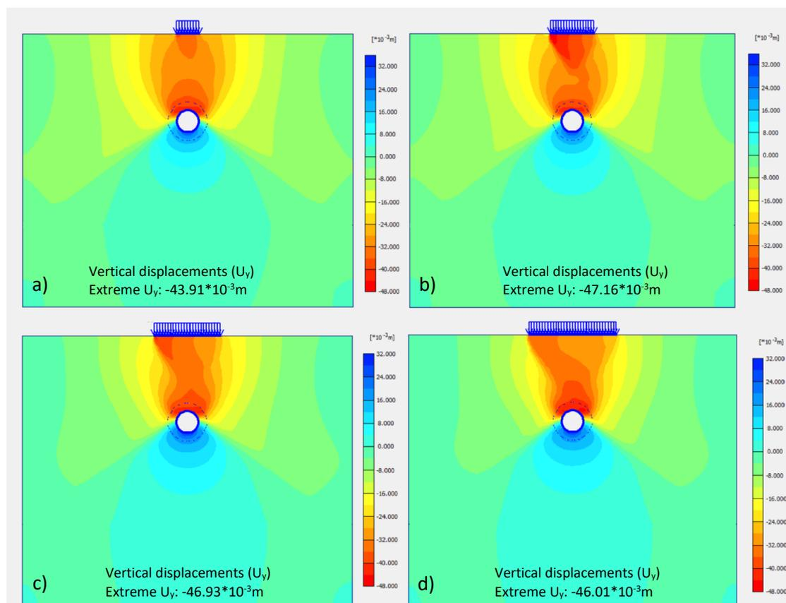
**Figure 11.** General presentation of vertical displacements ( $U_y$ ) a) for  $D=10$  m,  $H=25$  m,  $B=10$  m, b) for  $D=10$  m,  $H=25$  m,  $B=20$  m, c) for  $D=10$  m,  $H=25$  m,  $B=30$  m, d) for  $D=10$  m,  $H=25$  m,  $B=40$  m
