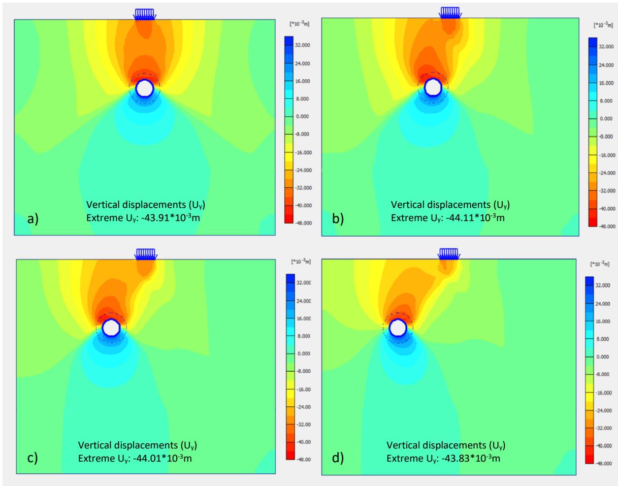
**Figure 9.** General presentation of vertical displacements ( $U_y$ ) a) for  $D=10$  m,  $H=25$  m,  $L=0$  m, b) for  $D=10$  m,  $H=25$  m,  $L=10$  m, c) for  $D=10$  m,  $H=25$  m,  $L=20$  m, d) for  $D=10$  m,  $H=25$  m,  $L=30$  m
