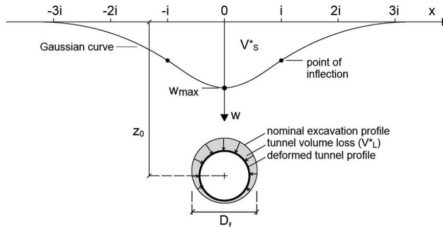
**Figure 2.** Gaussian curve for transverse settlement trough, nominal tunnel diameter, volume of the settlement trough,  $V^*_s$  and volume loss at the tunnel excavation profile,  $V^*_L$  (Ads et al., 2023).
