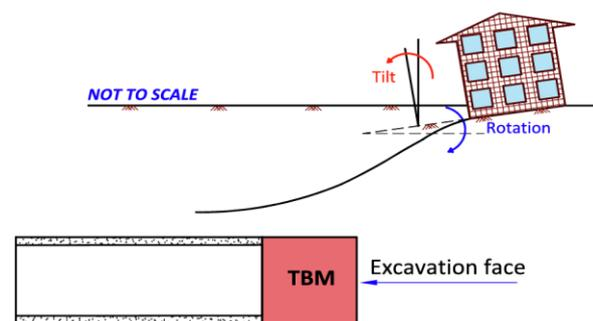
**Figure 1.** Complications to surface structures due to settlement (Ads et al., 2023)
