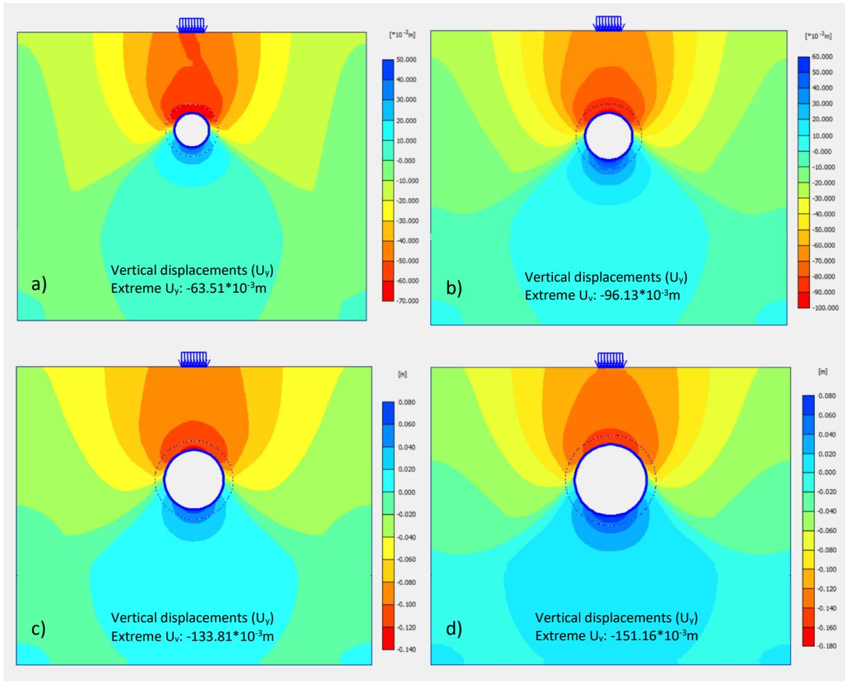
**Figure 7.** General presentation of vertical displacements ( $U_y$ ) a) for  $D=10$  m,  $H=25$  m, b) for  $D=15$  m,  $H=25$  m, c) for  $D=20$  m,  $H=25$  m, d) for  $D=25$  m,  $H=25$  m
