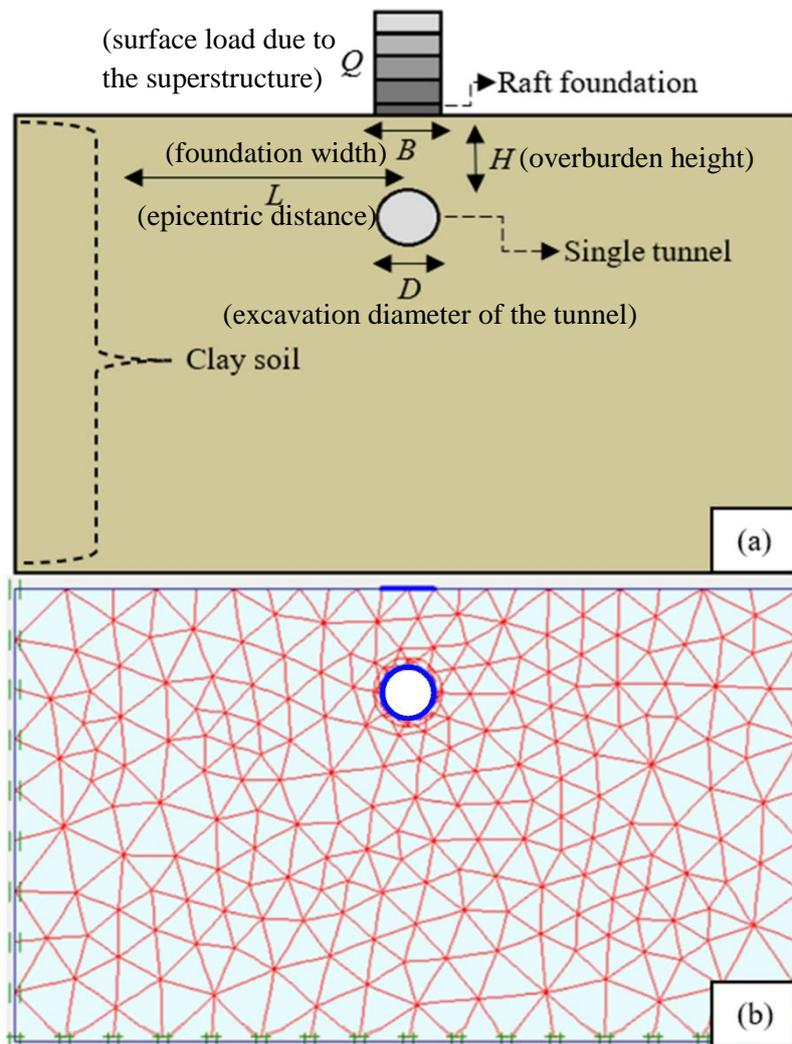
**Figure 4.** a) Geometric model b) Finite element network
