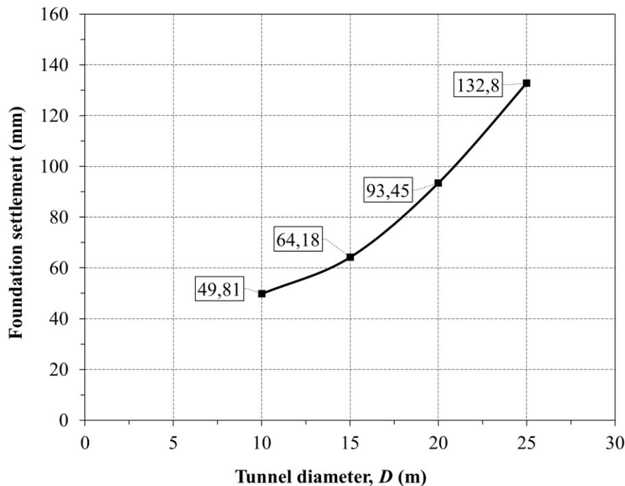
**Figure 8.** Tunnel diameter-foundation settlement curve
