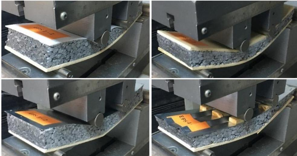
**Figure 3.** Four-point bending tests of EPS specimens
