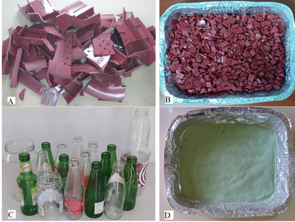
řekil 1. Atık sandalye paraları (A-B), atık cam řiřeler (C) ve öđütülmüř cam tozu (D) Figure 1. Waste chair parts (A-B), waste glass bottles (C) and ground glass powder (D)
