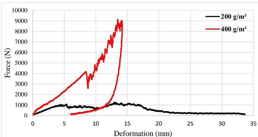
Figure 8. Effect of fiber weight on 50 Joule impact energy
