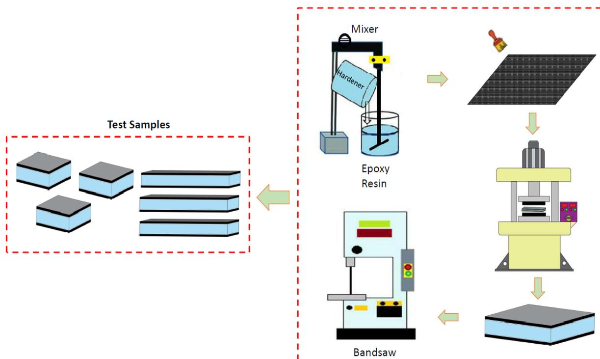
**Figure 3.** Schematic representation of the manufacturing process
