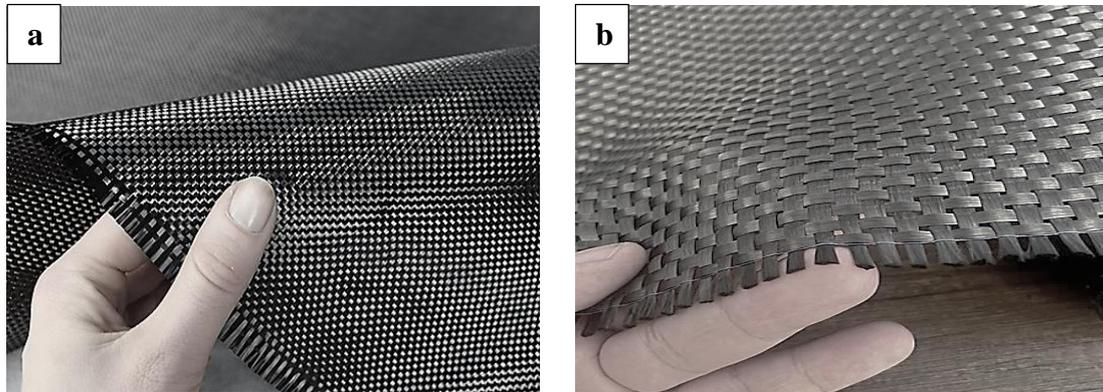
**Figure 2.** Carbon fiber woven fabrics used a) 200 g/m<sup>2</sup>, b) 400 g/m<sup>2</sup>
