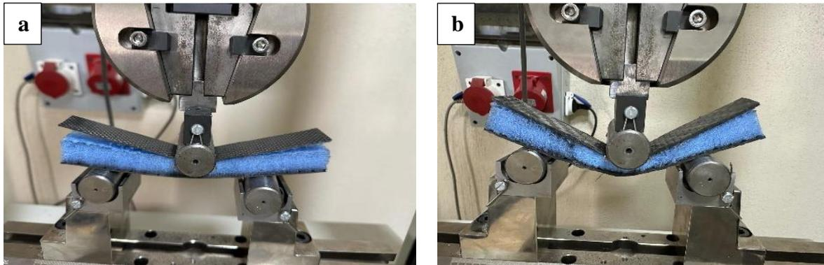
Figure 5. a) 200 g/m<sup>2</sup>, b) 400 g/m<sup>2</sup> Three point bending test
