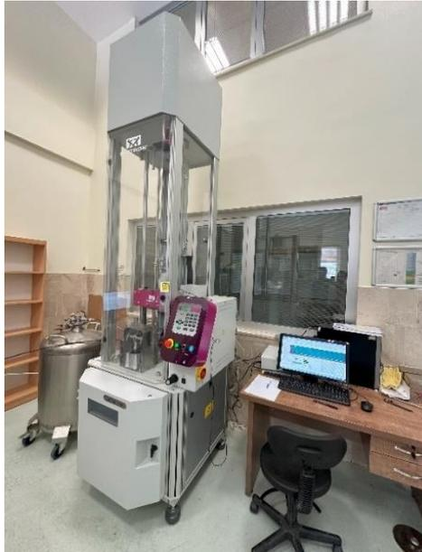
**Figure 4.** Low speed impact tester
