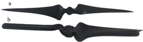
**Figure 3.** View of the printed propellers.
