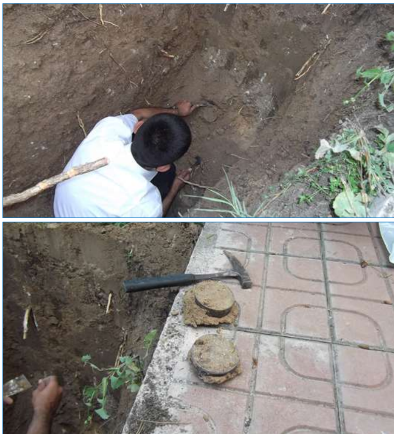
Fig. 12. Taking undisturbed samples from Trial pit-2
