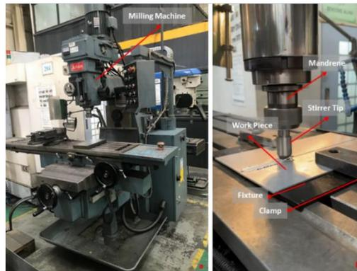
Figure 2. Milling machine (a), FSW application (b).
