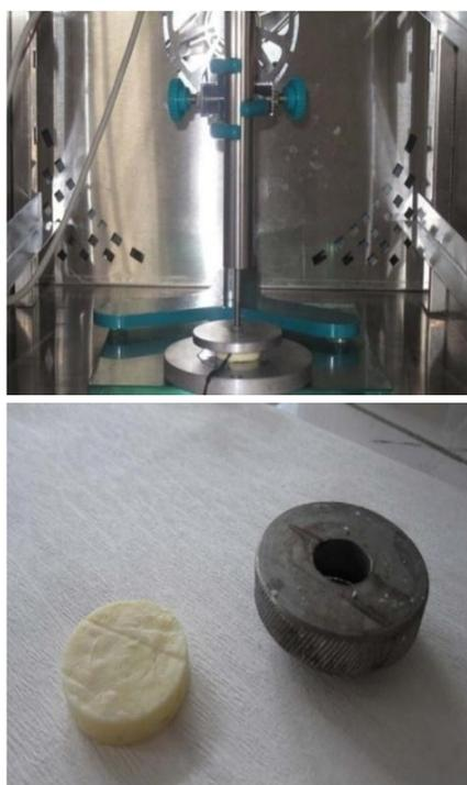
Figure 2. The designed melt profile device and the cut cheese sample.
