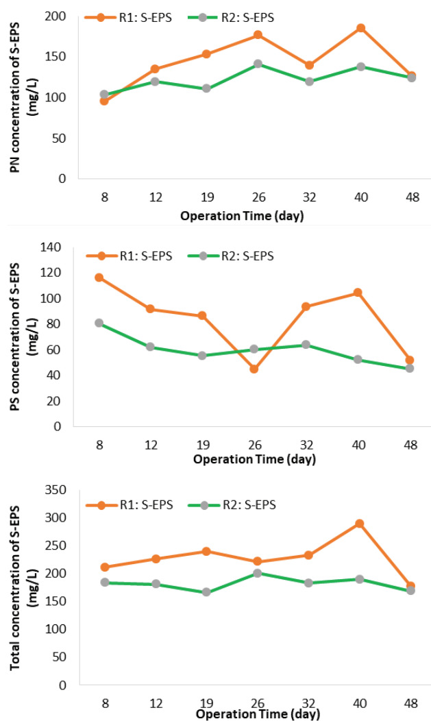
Figure 4. Variations of PN and PS concentrations of S-EPS throughout the MBR and GAC-MBR operation.
