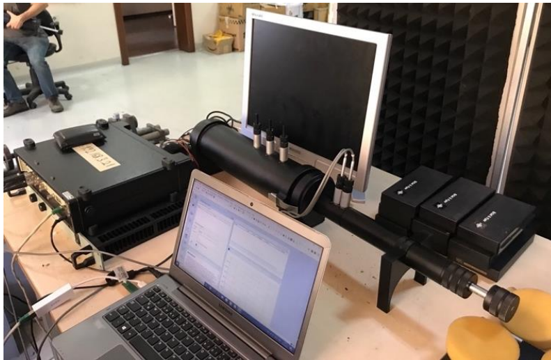
Fig. 3. Impedance Tube Assembly Used in Measurements (Özbek, 2022).
