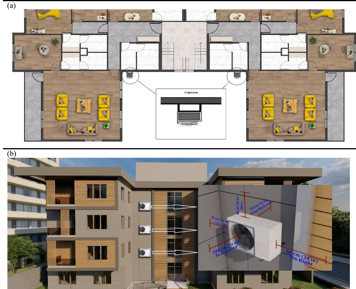
Figure 7. Precreated location in the building for the condenser of the AC ((a)-layout plan, (b)-exterior view).
