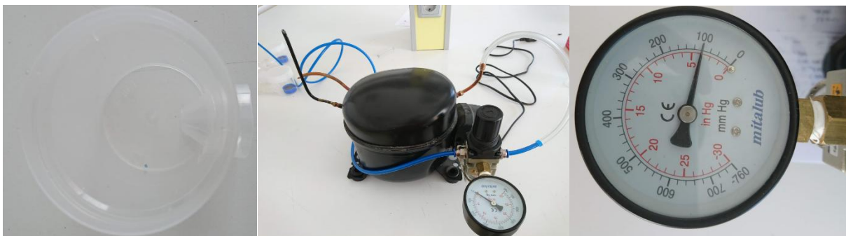
Fig 2 Lidded plastic container designed to be funnel-shaped for storing manures (left), the vacuum pump (middle), and vacuum pump's suction pressure (right)
