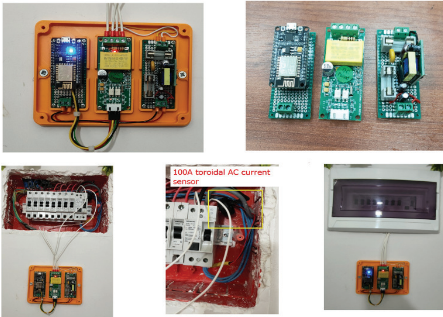
Figure 12. Installing AC smart plug in a real house. Measure the energy and analyze the consumption behavior.
