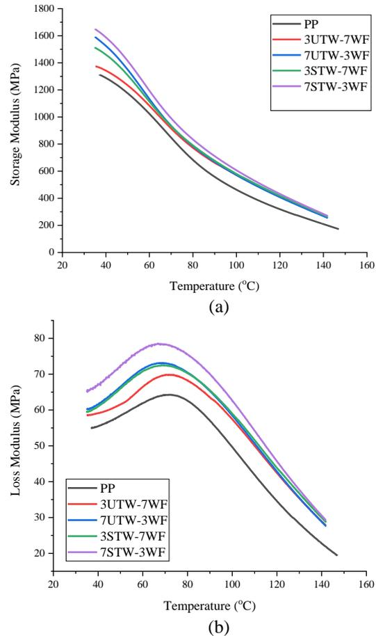
Figure 3. (a) Storage modulus and (b) Loss modulus
