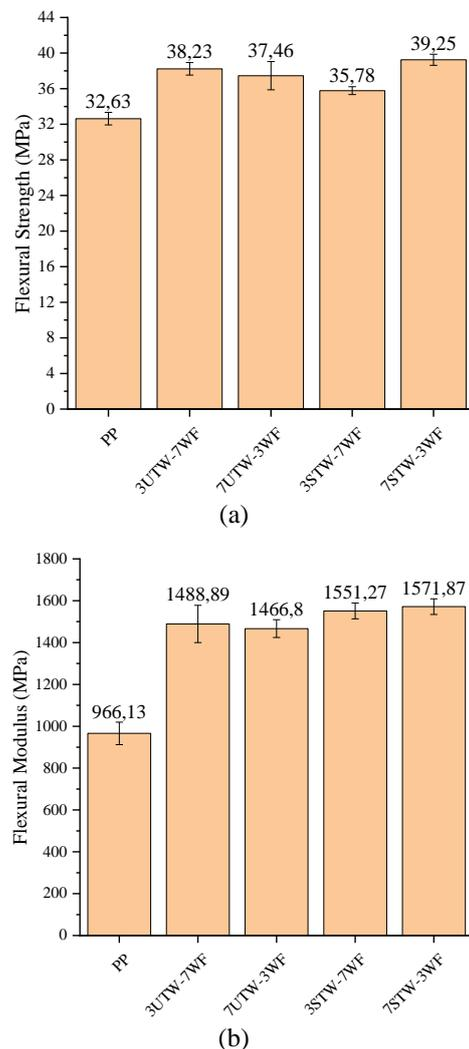
**Figure 2.** (a) Flexural strength and (b) Flexural modulus
