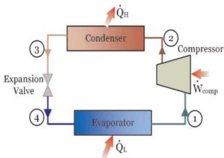
**Figure 1.** Vapor compression refrigeration system. (Seyam, 2019)
