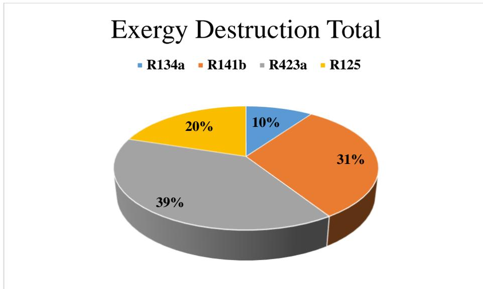
**Figure 4.** Distribution of exergy destruction rates of the refrigerants used in the system.
