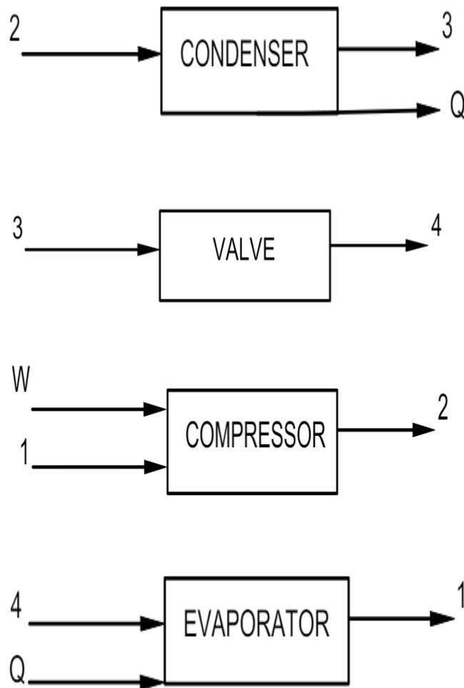
**Figure 2.** Schematic diagram of the components of the vapor compression refrigerant system.
