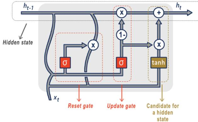
Figure 6. Schematic Representation of the GRU Cell and Its Gating Mechanisms
