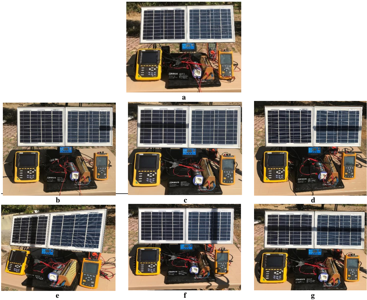
Figure 4. Shading effect test system.
