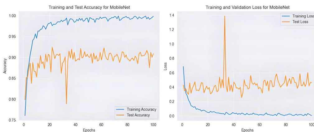
Figure 5. Training and Test Accuracy/Loss graphs for MobileNet according to the number of epochs
