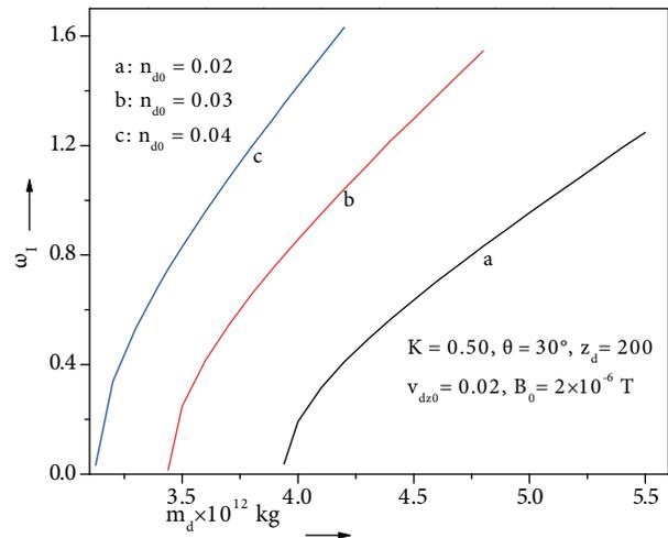
**Figure 2.** Growth rate of instability plotted as a function of the dust mass  $m_d$  for different values of dust number density  $n_d$ .
