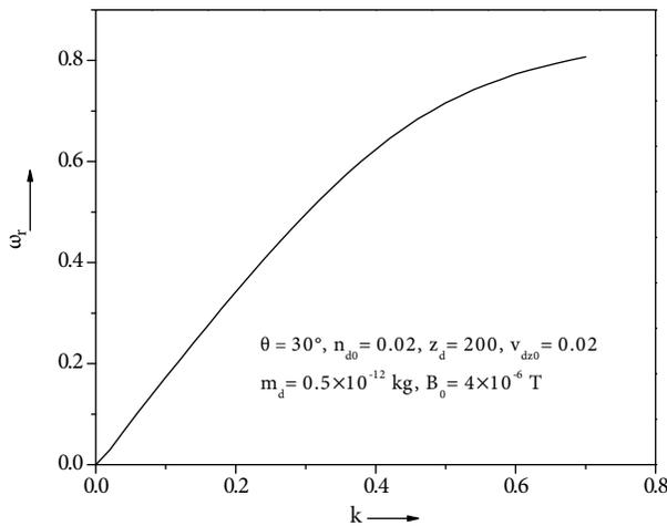
**Figure 1.** Dispersion curve for dust acoustic wave.
