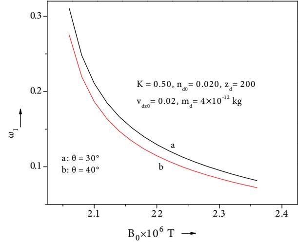
**Figure 4.** Dependence of the growth rate of instability on the strength of magnetic field  $B_0$  and the angle of propagation  $\theta$ .
