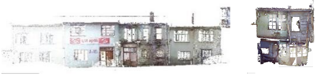
Figure 2. Laser Scan Data - scans of plan and section (created by the author).
