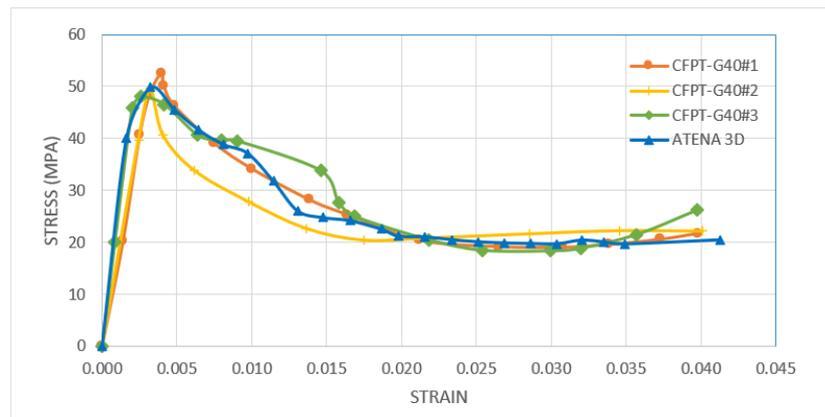
Figure 4. Comparison of reference models and FEM model (Topal, 2022)
