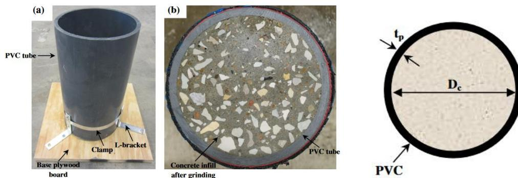
**Figure 2.** Specimen preparation (a) PVC tube before casting; (b) ground end. (Fakharifar and Chen, 2017)
