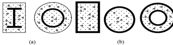
**Figure 1.** Composite columns with various types (a) Encased and (b) concrete-filled. (Abbas, 2023)
