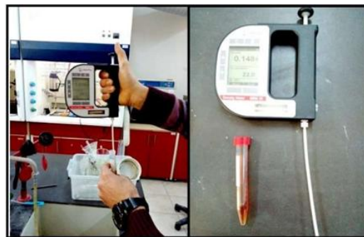
Figure 4. Measurement of H. perforatum extract liquid density
