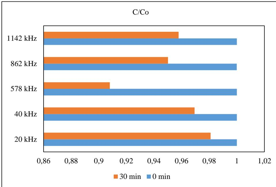
**Fig.2.** The ultrasonic oxidation of MC-RR with different frequencies (MC-RR=1.25 µg/L, pH=6.75, T=20 °C, t=30 dak)
