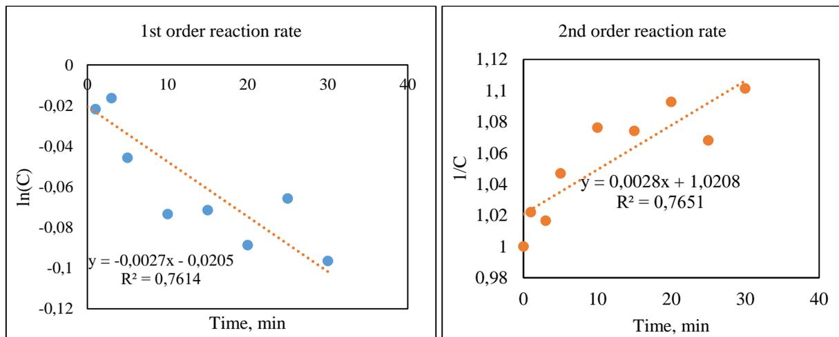
**Fig.3.** The concentration reduction of MC-RR by ultrasonic oxidation with 578 kHz frequency.
