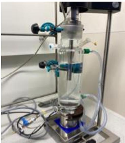
**Fig.1.** The ultrasonic reactor with low and high frequencies.
