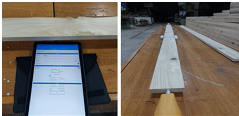
Figure 3: Determination of strength classes of timber by acoustic test device
