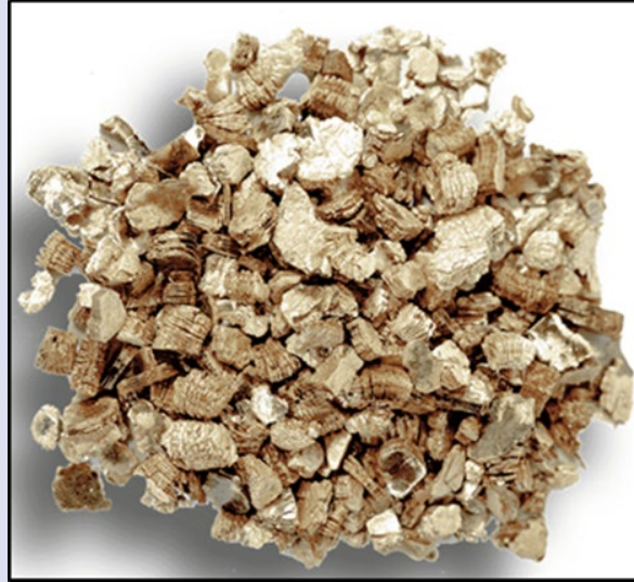
Figure 4. Trade name "Coarse Vermiculite" used in the experiment.
