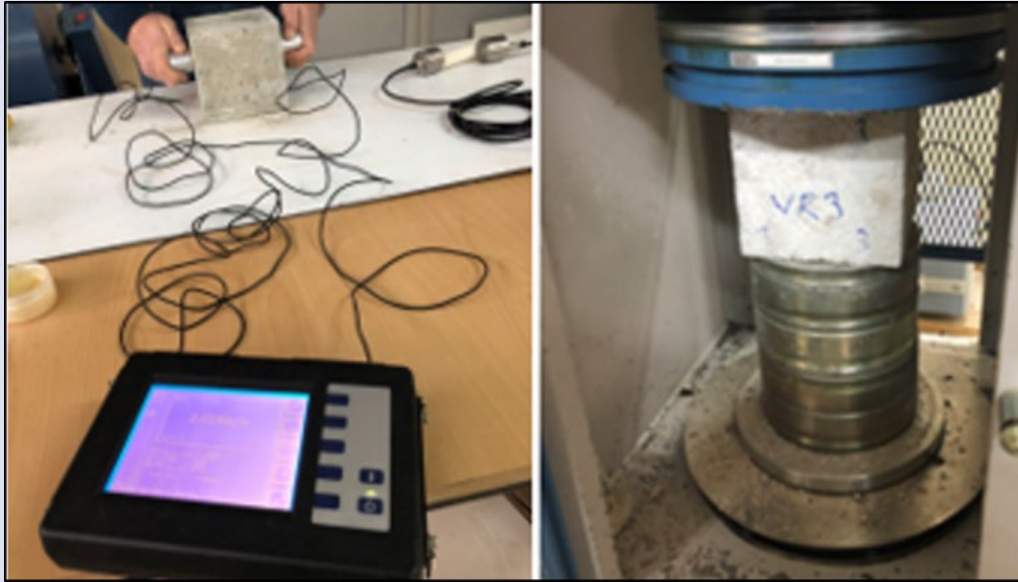
Figure 6. P-wave ( V_p ) velocity measurement and compression test of cubic specimens
