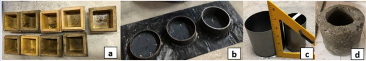
Figure 5. Sample molds to be used in the experiments. (a) cubic molds, (b) cylindrical molds, (c) cylindrical vase molds and (d) cylindrical vase.
