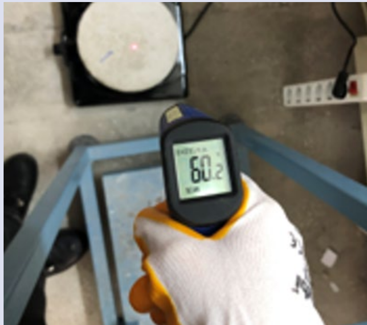
Figure 6. Temperature transition test for cylindrical specimens
