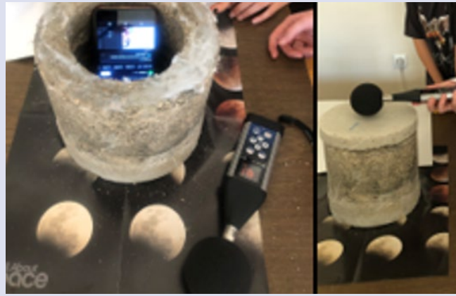
Figure 7. Sound transmission experiment. Internal and external sound measurement
