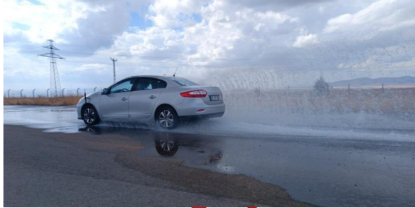
Şekil 7. Asimetrik desenli lastik aquaplaning testi (Asymmetrical pattern tire aquaplaning test)
