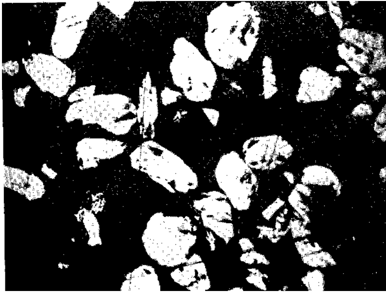
Photo 10 — (Magnification: 80 X) Polished surface containing a Bursaitite concentrate (Blende (grey) which remained scantily is seen as mixed grains)
